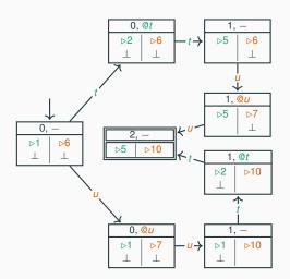
Tracking every statement can lead to large state diagrams. We can simplify a diagram by skipping lines irrelevant to concurrent behavior.
